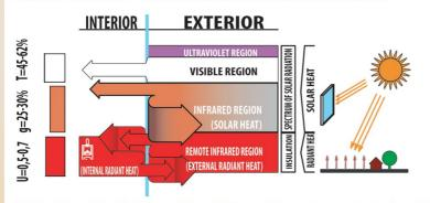
High insulating ability with slight regulation of light transmission and suppression of solar radiation
